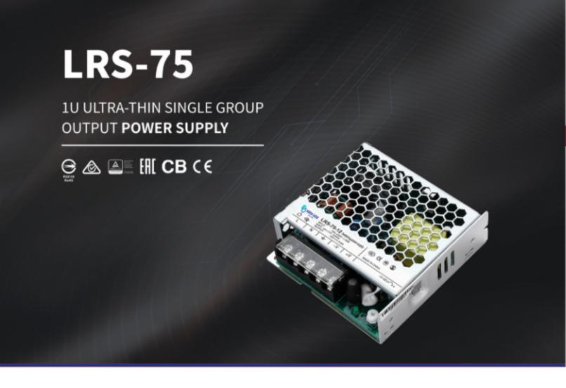
The LRS-75 series is a 75W single group output enclosed power supply with a 30mm low profile design and a full range of AC inputs of 85 to 264VAC. The entire series provides 5V、12V、15V、24V、36V、and 48V output.
